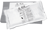
POTTING COMPOUND — PC21 Re-enterable potting compound which pours yellow and cures transparent so connections are easily located. It meets NEC requirements for potting junction boxes and is recommended as part of the installation in areas with high water tables, poor drainage or are prone to flooding to protect the junction box from water intrusion. Sold separately.
