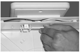
4. Lay cam locking pin between canopy posts and snap into retaining hooks. Rotate cam locking pin up to lock into place.
