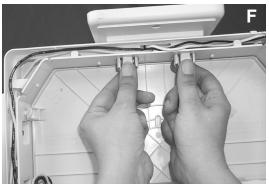
**To Remove Canopy-**Rotate cam locking pin level with housing and remove from hooks. Squeeze snaps and pull housing free.
