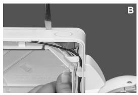
**To Remove Back Plate-**Press in snaps at bottom or top of housing. Then release latches A and B from the inside of housing.
