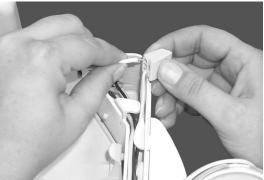
5. In upper right corner of housing wire channel connect input leads using pushnuts and jumper wire provided to route wires to j-box. Connect battery and snap face plate onto housing. Remote lamp option: Connect remote lamps to yellow and blue wires using pushnuts and jumper wire provided to route wires to j-box.
