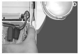
Remove and Relocate Lamp Mount Assembly Remove face plate and back plate. Disconnect lamp harness from lamp board. Press four snaps (two each side) to release lamp mount assembly from housing. Relocate to top of housing and resnap into place. Connect lamp harness to lamp board.
