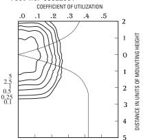
1000W metal halide lamp 107,800 rated lumens. Footcandle values based on 35' mounting height, distribution Type V, cutoff.
