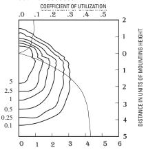
1000W high pressure sodium lamp, 140,000 rated lumens. Footcandle values based on 35' mounting height, distribution Type IV, cutoff.
