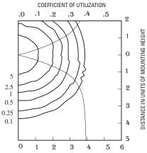
1000W high pressure sodium lamp, 140,000 rated lumens. Footcandle values based on 35' mounting height, distribution Type V, cutoff.
