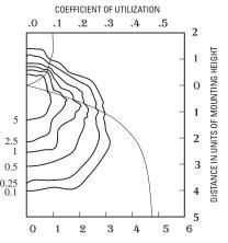
1000W metal halide lamp 107,800 rated lumens. Footcandle values based on 35' mounting height, distribution Type IV, cutoff.
