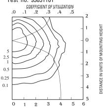
1000W high pressure sodium lamp, 140,000 rated lumens. Footcandle values based on 35' mounting height, distribution Type III, cutoff.
