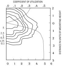
1000W metal halide lamp 107,800 rated lumens. Footcandle values based on 35' mounting height, distribution Type III, cutoff.
